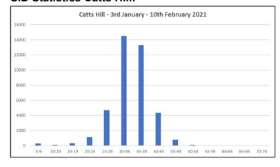
Throughout January and early February SID was deployed on Catts Hill to monitor the traffic on that part of the B2100.
